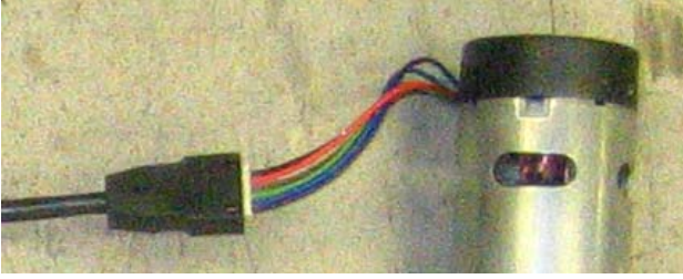
Correctly connected motor
